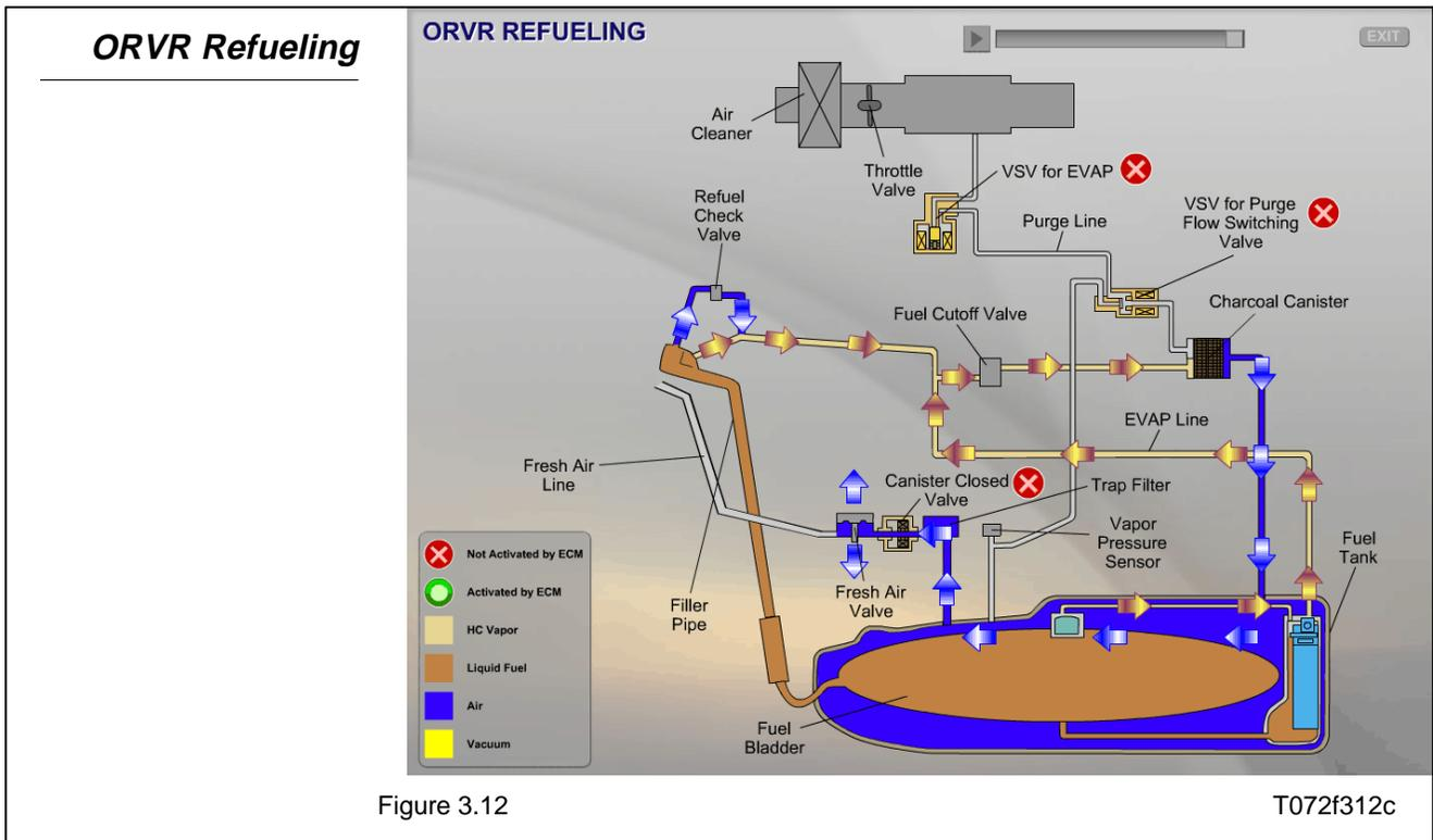
**Purging** During normal purge operation the engine is running and the ECM duty cycles the EVAP VSV ON and OFF, allowing vacuum from the intake manifold to pull air through the EVAP system. The Purge Flow Switching Valve is OFF, opening the connection between the charcoal canister and the EVAP VSV. HC vapor flows from the charcoal canister to the EVAP VSV and into the intake manifold.
