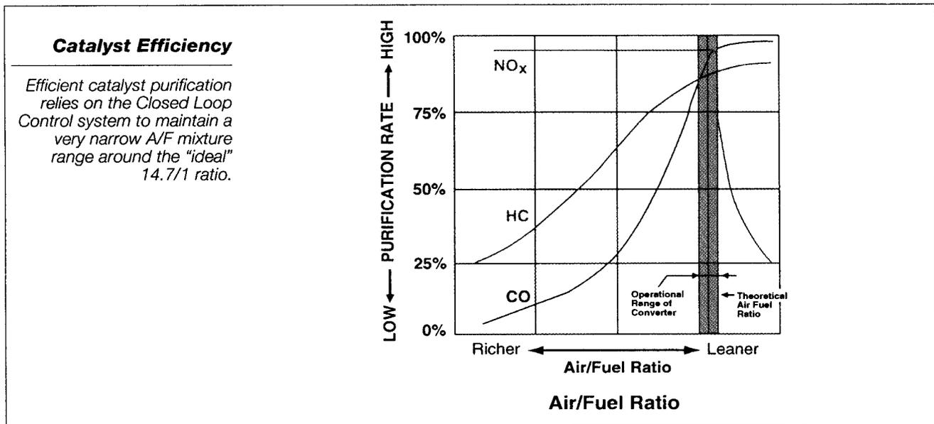
As mentioned in the beginning of this section, precise closed loop control relies on accurate feedback information provided from the exhaust oxygen sensor. The sensor acts like a switch as the air/fuel ratio passes through stoichiometry.
