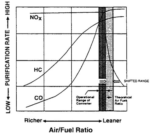
It is often difficult to identify a sensor which is marginally degraded, and in many cases, vehicle driveability may not be effected significantly. With the advent of IM240 emissions testing, however, marginal sensor degradation may cause some vehicles to fail the NOx portion of the loaded mode test.
