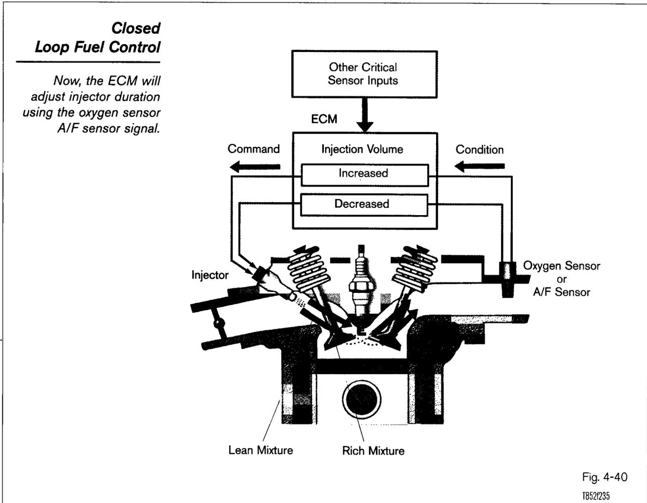
**Closed Loop Operation/Oxygen Sensor**
