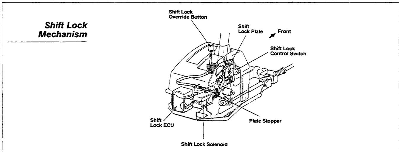
The shift position switch (shift lock control switch) is used to detect the position of the shift lever. It has two contacts, P1 and P2. When the select lever is in the Park position, P1 is on (closed) and P2 is off (open). In this position, the key can be removed but the select lever is locked in position.
