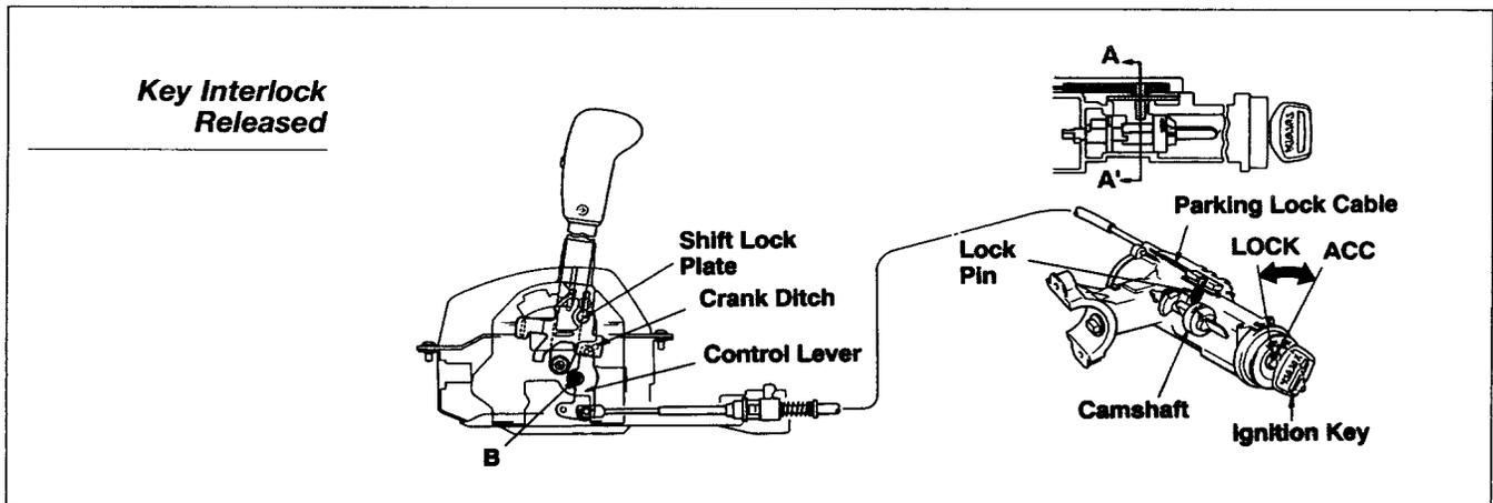
When the shift lever is in the Park position, the control lever rotates around B counterclockwise, pushing the parking lock cable so that the lock pin does not interfere with the camshaft. In this position, the key can be turned to the Lock position and removed.
