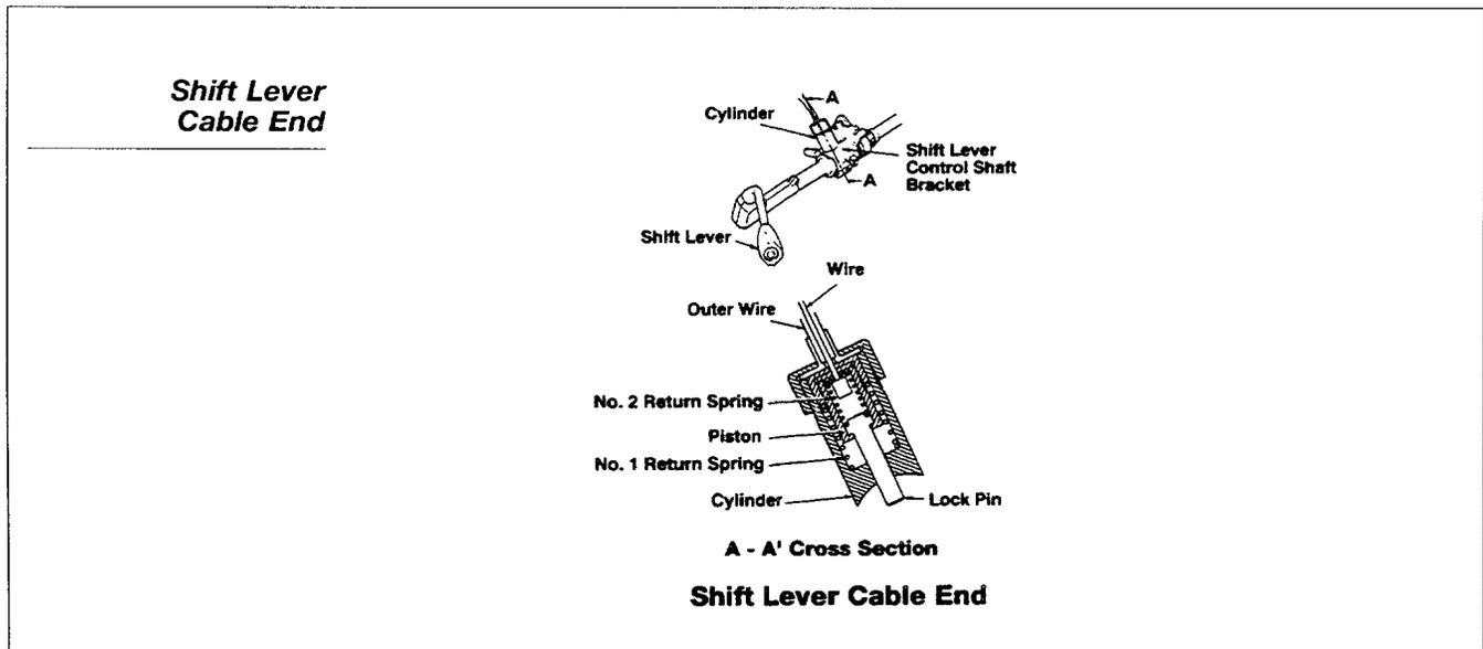
When the shift lever is in the Park range and brakes are not applied, the cable compresses the No. 1 return spring and pushes the lock pin engaging the round hole in the inner shaft, locking the shift lever in Park
