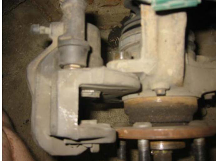
The four piston calliper, due to its size is mounted on the other side of the hub. This means that the calliper is drilled while the ST205 hub is tapped.
