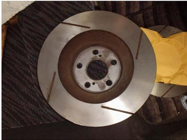
ST205 disc after being machined down to 300mm
